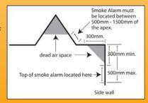
If it is not practical to install the smoke alarm on the ceiling, then it may be installed on the wall between 300mm to 500mm below the ceiling.
